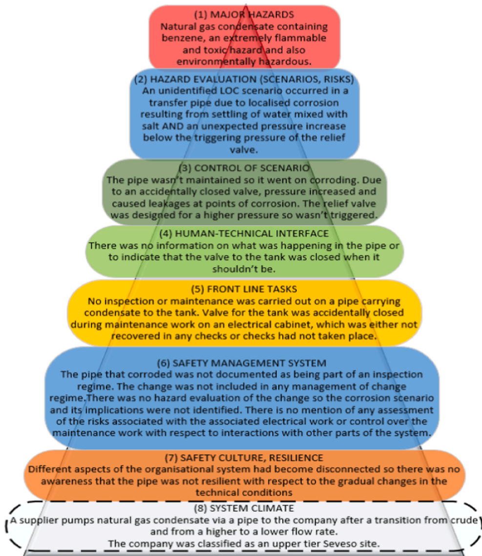
Fig. 9. Example of a Dutch material degradation accident from 2010, portrayed as a slice of the holistic model.
