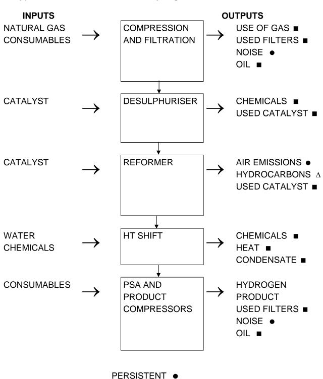
Appendix 3: Emissions or Waste – Hydrogen and Carbon Monoxide Plant
