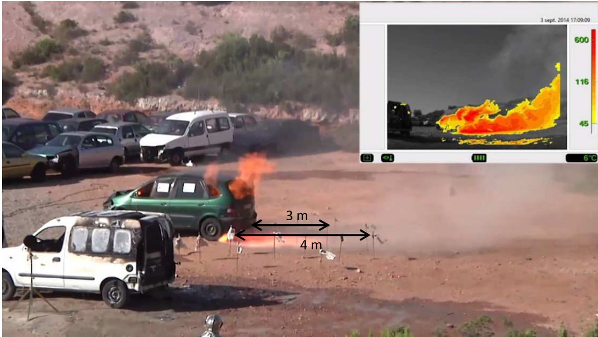
Figure 4: Jet fire exiting from a TPRD mounted on a 700 bar H 2 tank
