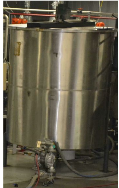
Figure 4. Exemplar AB Specialty batch tank with agitator and lid. (Credit: AB Specialty)
